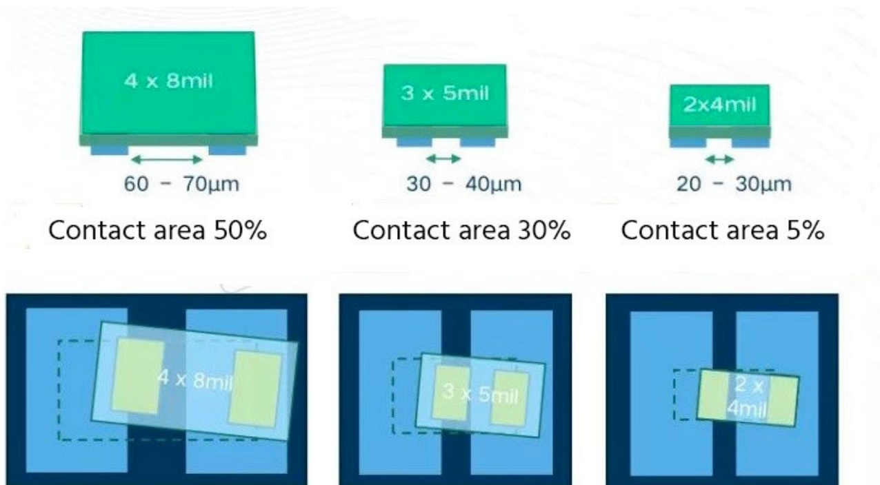
Figure 1: With the same deviation, the effective soldering area has been reduced from 50% to 5%. (Source: ASM Pacific)
